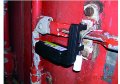
The simplest type of electronic seals contains only a seal ID number. The most common technology for such an eSeal is passive RFID (Radio Frequency Identification), which requires an appropriate reading device and software.
