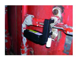
The simplest type of electronic seals contains only a seal ID number. The most common technology for such an eSeal is passive RFID (Radio Frequency Identification), which requires an appropriate reading device and software.
